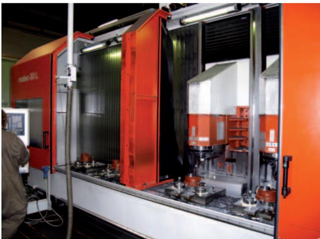
Fig. 1. Chucking on the left, machining on the right – handling two parts at the same time: the two-station Matec 30 L machine with two traversing columns allows the Aerzener Maschinenfabrik to perform the economical machining of castings in short runs with minimal non-productive times.
