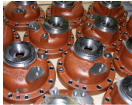
**Fig. 4. Housing cover made from a mass produced casting – machining to a finish takes place in a single chucking through the casting scale from above; relief-turning the recess poses no problems.**
