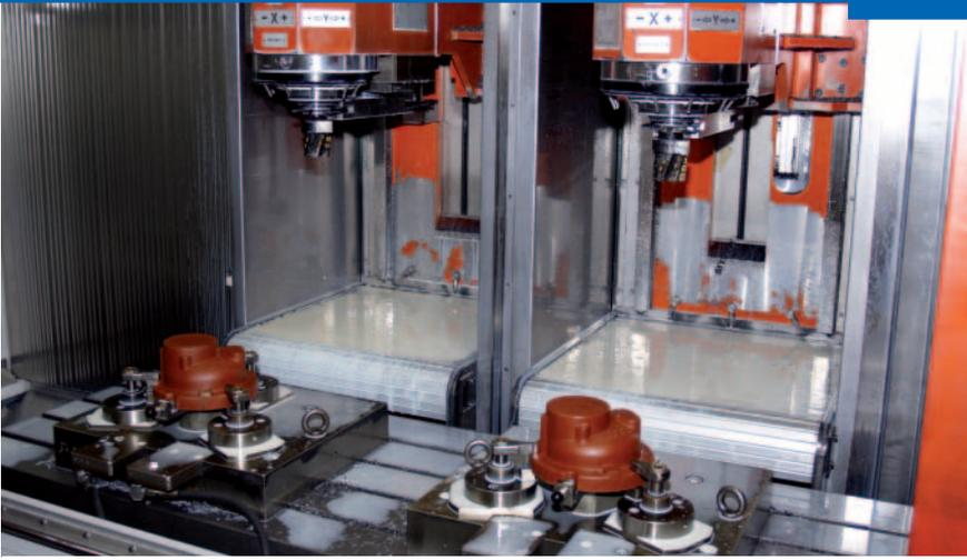
**Fig 5. Electronically linked twin spindles - the Aerzener Maschinenfabrik benefits in several ways from the machine designed by the manufacturers, Matec, in the form of flexibility, quality and economy.**
