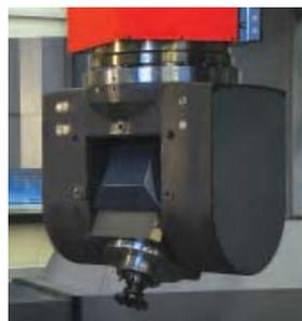
2-axis NC motor spindle milling head
