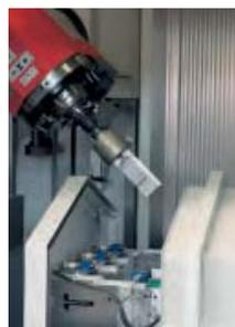
NC gripper depositing a work part
