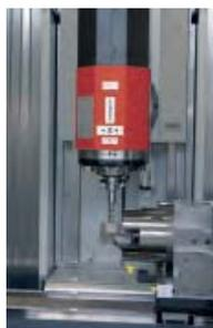
Machining on counterspindle
