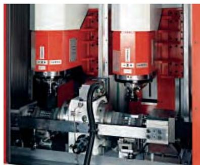
Left-sided working area with clamping device
