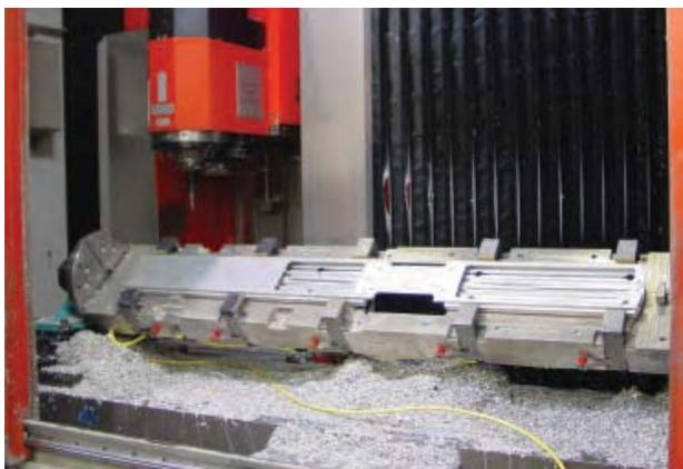
Swiveling device for clamping of extremely damageable hollow chambered rails
